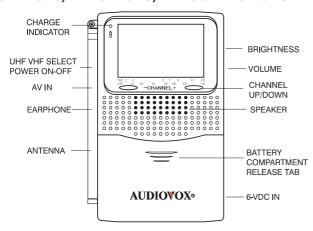
**Charge indicator:**Illumlinates when battreries are charging **UHF/VHR Select/Power On/Off:**Turns power on and off;Selects UHF/VHF TV band
